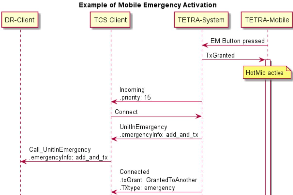
**Figure 26 – MSC for Unit in Emergency**
