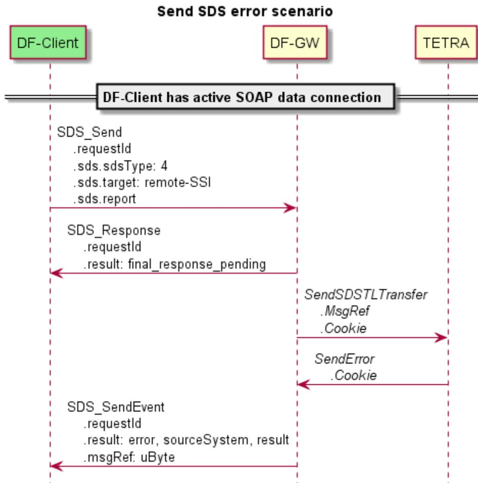
Figure 28 – MSC Send SDS error scenario
