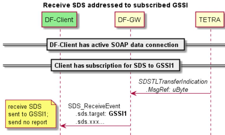
**Figure 30 – MSC Receive SDS addressed to subscribed GSSI**
