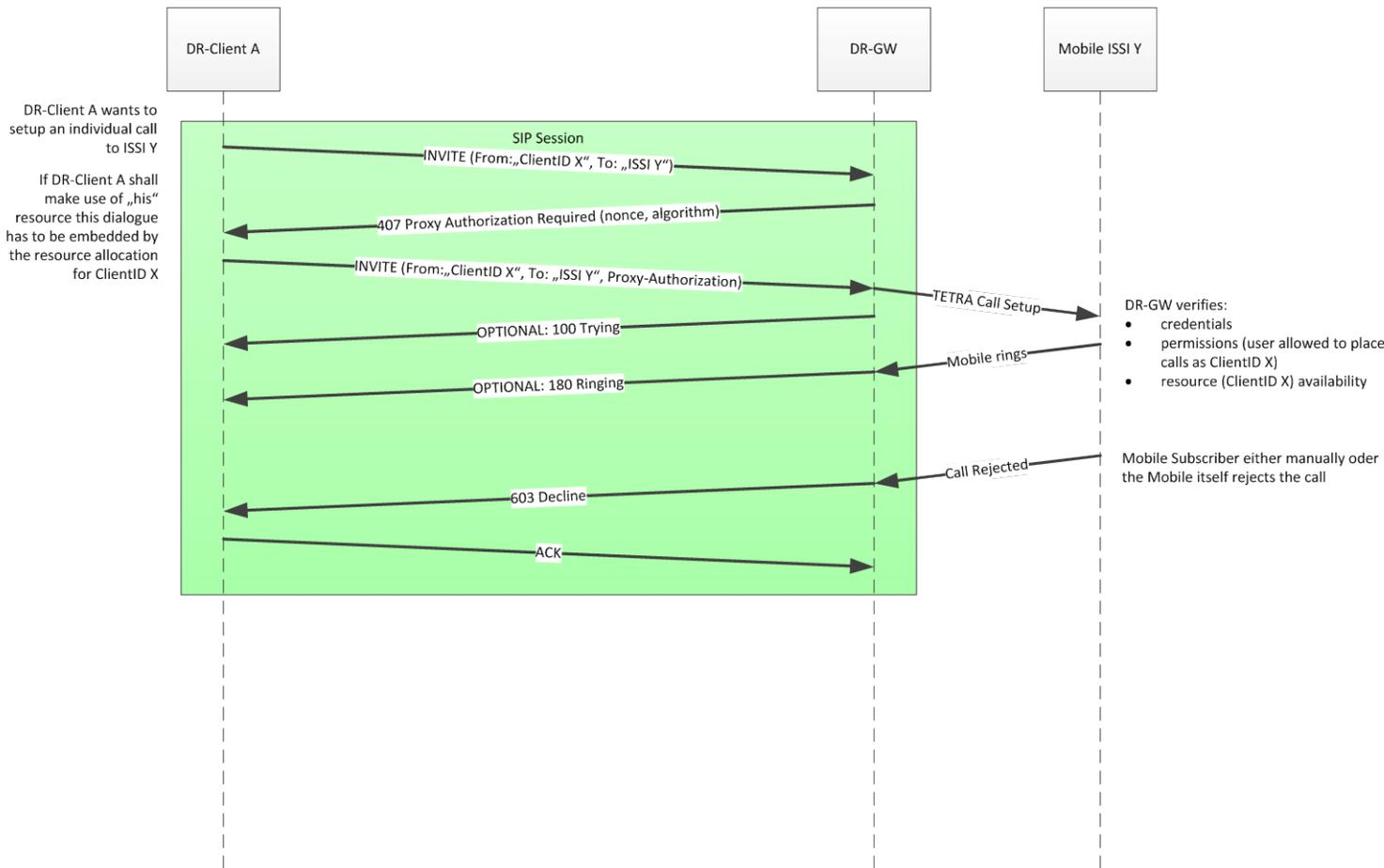
**Figure 9 – MSC for GW Rejected Outgoing Individual Call**
